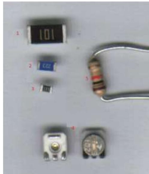
1, 2 and three are examples of surface mount devices. 4 are typical examples of potentiometers. 5 is the typical example of a carbon film type resistor which the general hobbyist would use for a home / prototyping project.
