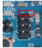
The power configuration requires that 1 set of jumper pins be closed. Shown on the image below, closing the jumper shown will enable the PCB to run at 5 Vdc.
